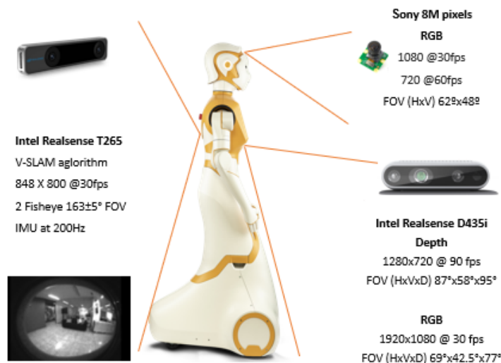
Figure 19 TIAGo robot: different components.
